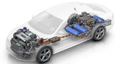
fuel cell system
