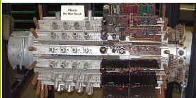
Mercury delay-line memory of UNIVAC 1000 words – 12 characters per word (1951)
